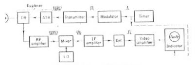
Fig. 1.3. Block diagram of a pulse radar.
